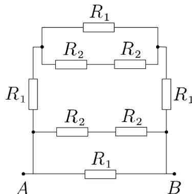
$$\frac{1}{R} = \frac{1}{R_1} + \frac{1}{2R_2} + \frac{1}{R_1 + R_1 + \frac{R_1 2R_2}{R_1 + 2R_2}}$$
